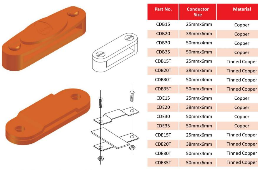
This ABRE DC Tape and Flat Clip suitable fix copper or tinned copper tape conductors and material made from high quality copper and aluminium alloy or tinned. And installation fixing with countersunk woodscrew 1 1/2" x no.10 and wall plug, used DC and Flat Type to meet IEC 62561-4.
